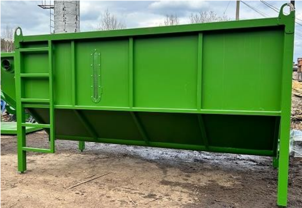
Picture 1. Storage hopper
